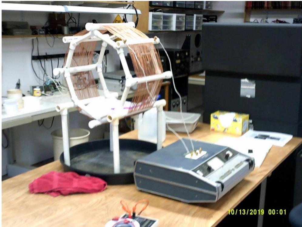
Figure 2 - PVC cage inductor.
