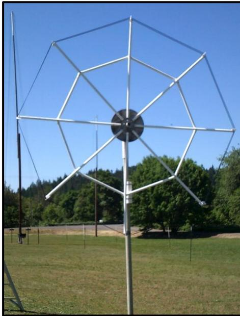
Figure 6 - Octagonal test loop.
