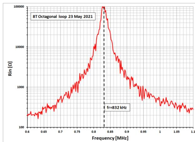
Figure 7 - Input resistance ( $R_{in}$ ) for an 8T octagonal loop.
