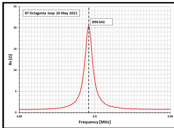
Figure 9 -  $R_s$  of the sampling loop.
