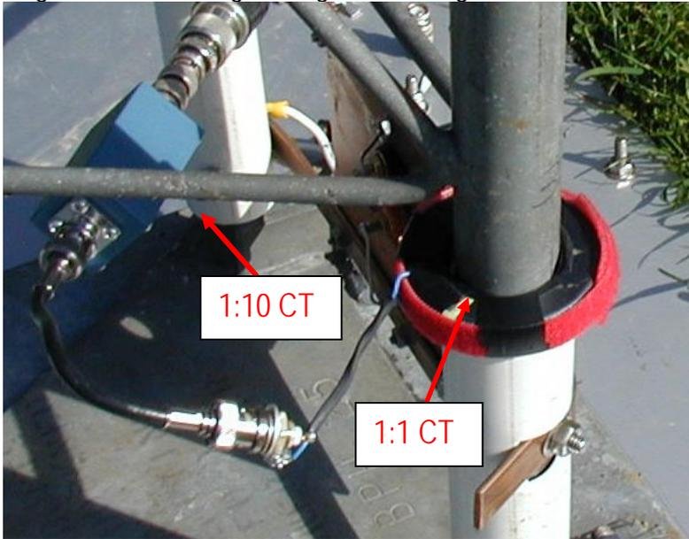
There is another CT shown in figure 7. That's the blue box. In the box there is a small 1:10 CT with BNC connectors at either end. I felt this approach was more flexible than winding more turns on the large CT. By using an auxiliary CT I can make up several with different turns ratios to suit the occasion and simply connect the one I want or go straight to the primary of the 1:1 CT around the tower leg.
