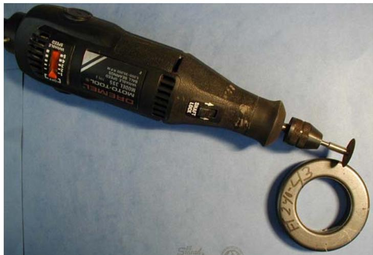
Figure 2, using a Dremel tool to cut the core.
