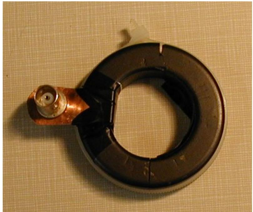
Figure 6, final assembly of the CT.
