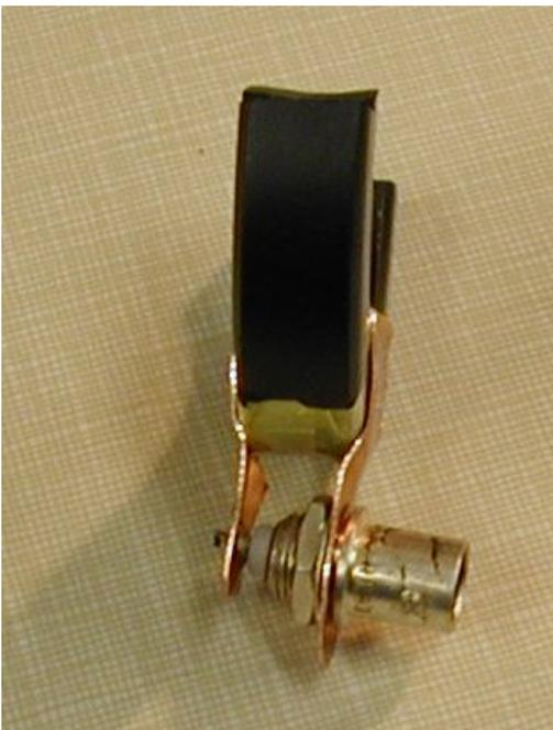
Figure 5, one turn secondary winding.
