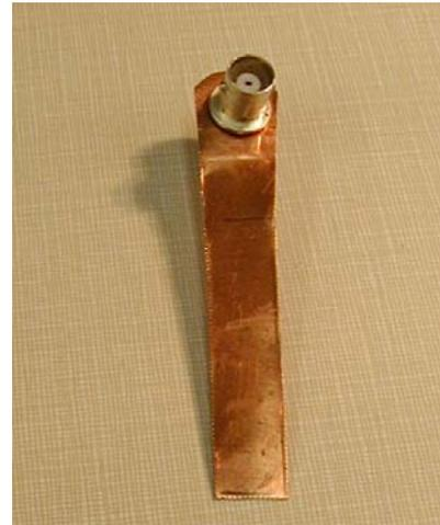
Figure 4, secondary winding.
