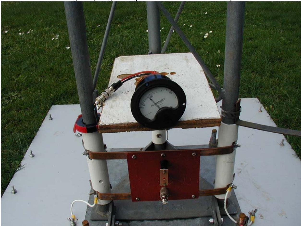
Figure 10, tower leg current when excited from nearby vertical.
