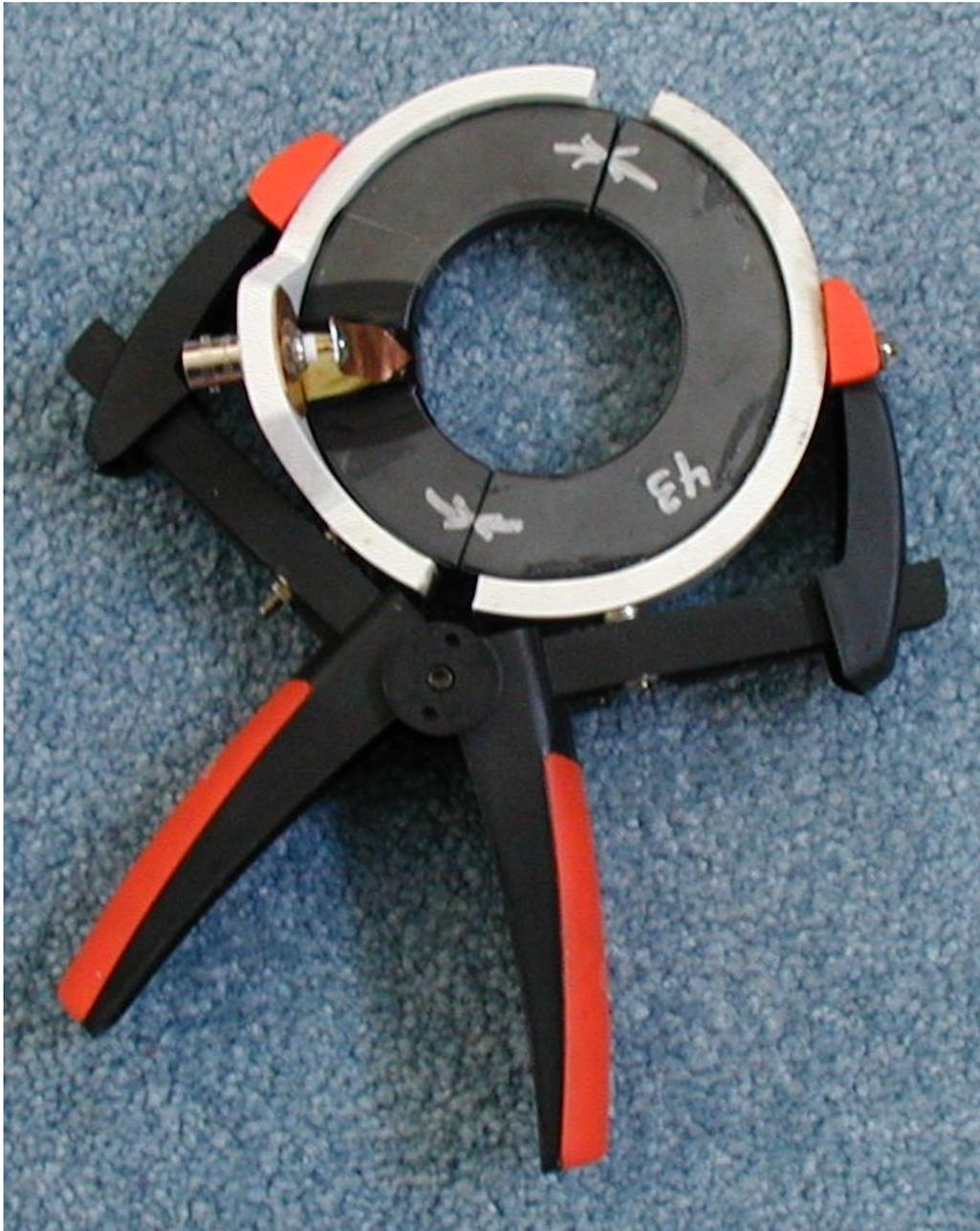
Figure 11, clamp-on current transformer.
