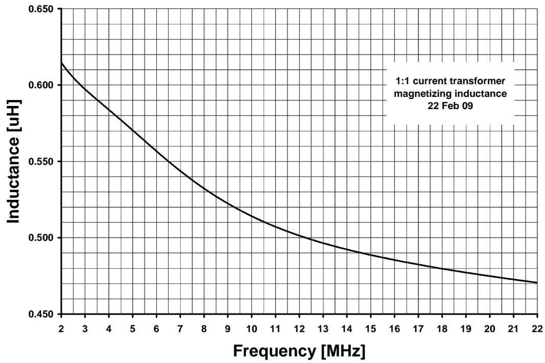
Figure 9, magnetizing inductance on the secondary.
