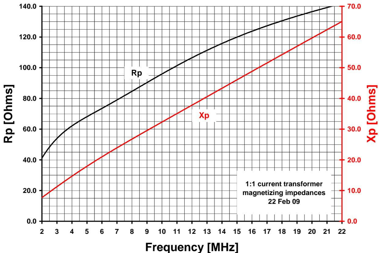
Figure 8, parallel resistance (Rp) and reactance (Xp) for the large 1:1 CT.
