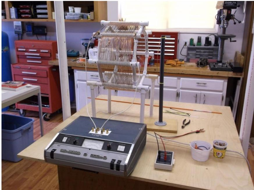
Figure 1 - Test inductor and experimental arrangement.
