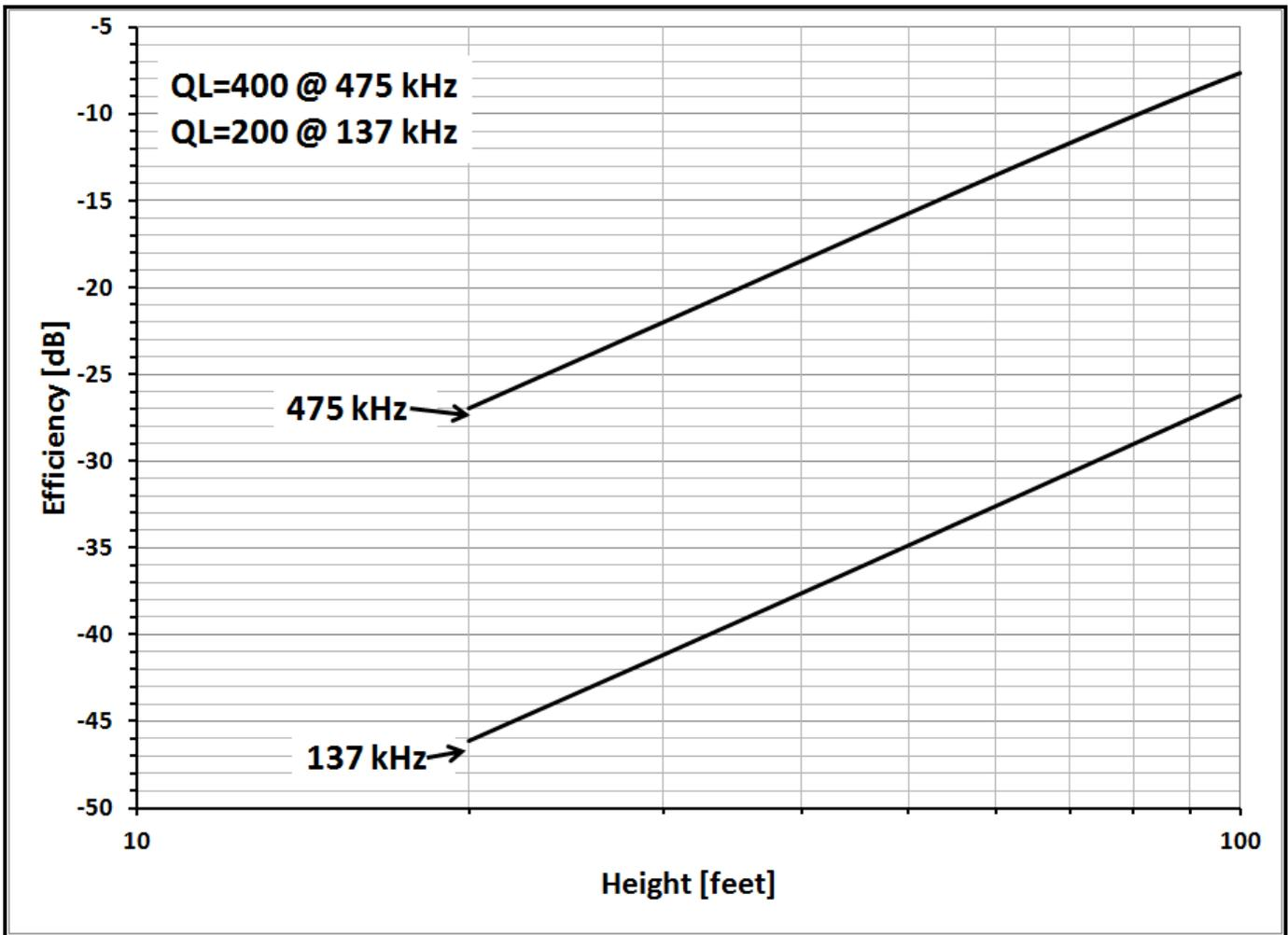
Figure 2.13 - Efficiency stated in  $\text{dB} = 10 \text{ LOG}(\text{efficiency})$
