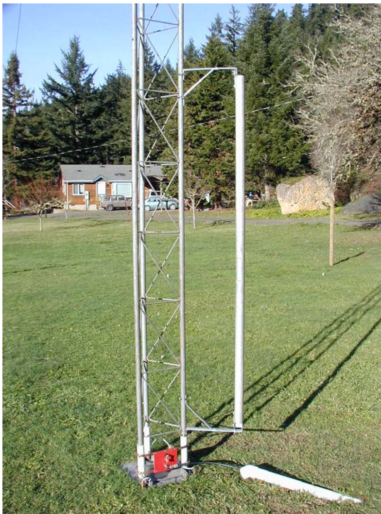
Figure 2, view of the shunt loop at the base of the test tower (28' of Rohn 25G).
