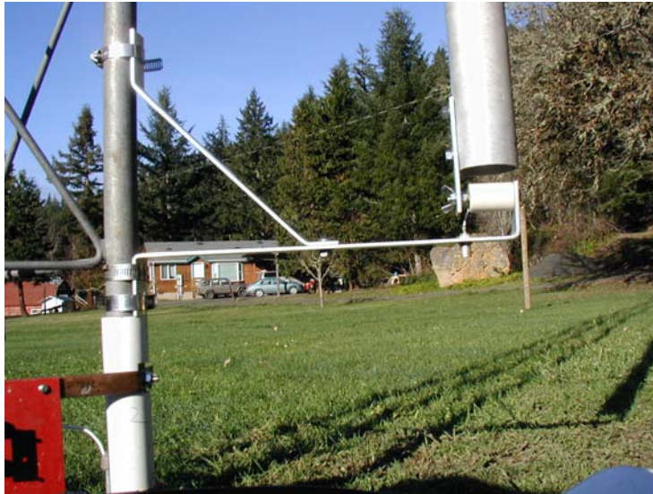
Figure 2, close-up of the bottom of the shunt wire showing the insulator and the BNC connector where the VNA is connected.
