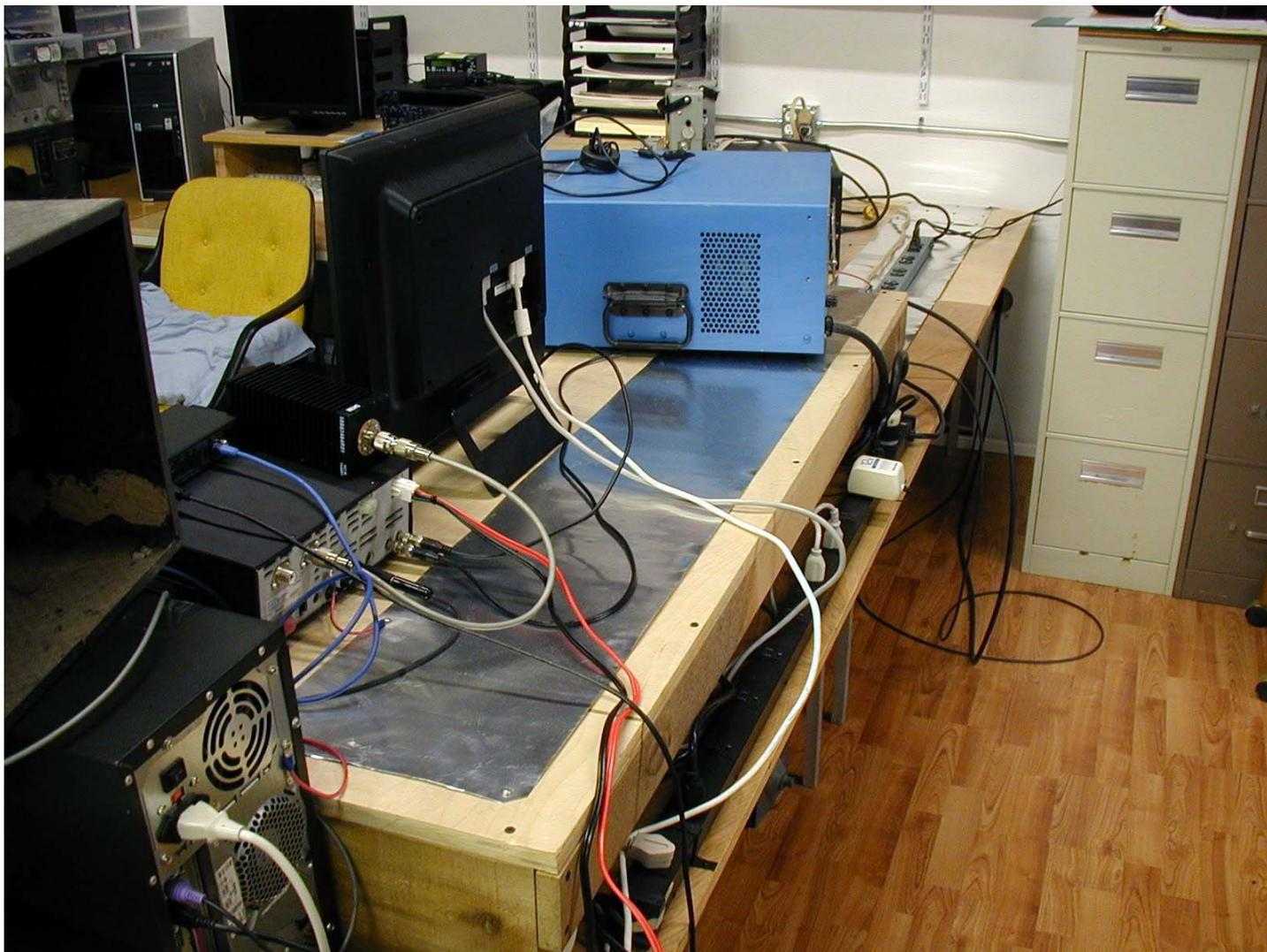
Figure 9, grounding strip inside the shack.
