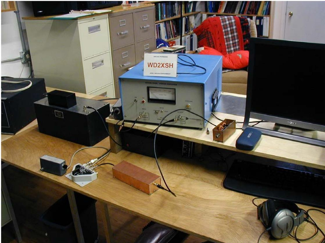
Figure 3, ENI 1040L amplifier and filters.
