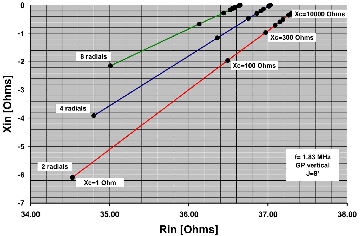
Figure 2 –  $Z_{in} = R_{in} + j X_{in}$  for different values of choke reactance ( $X_c$ ).
