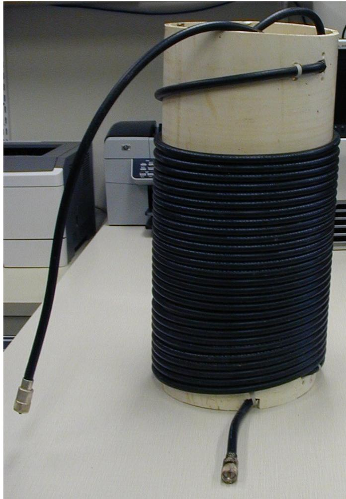
Figure 4, example of a 160m coaxial common mode choke.
