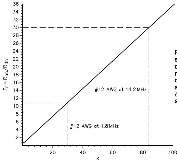
**Fig 1— $R_{ac}/R_{dc}$  ratio for solid round wire. Wire diameter ( $X$ ) is normalized to the skin depth,  $\delta$ , where  $d$  is the actual wire diameter and  $\delta$  is the skin depth in the same units.**
