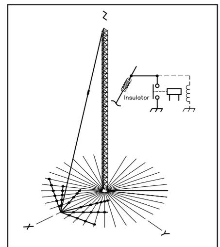
Figure 6—A simple 2-element slant-wire parasitic array.
