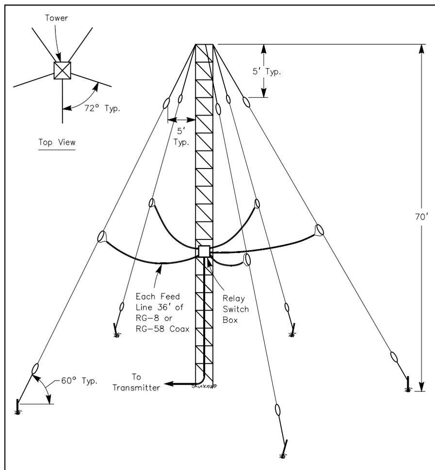
Figure 1—The K1WA Sloper System uses five identical one-half wavelength sloping dipoles spaced uniformly around a tall mast. Each feeder has an electrical length of about 135 degrees.
