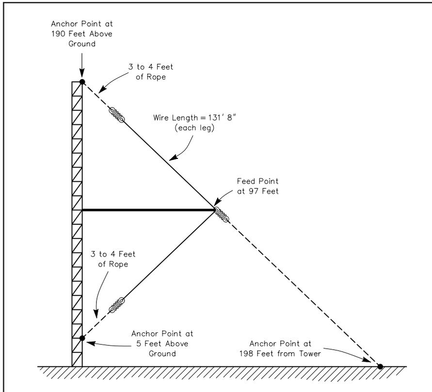
Figure 4—K3LR/K8UR bent element example.
