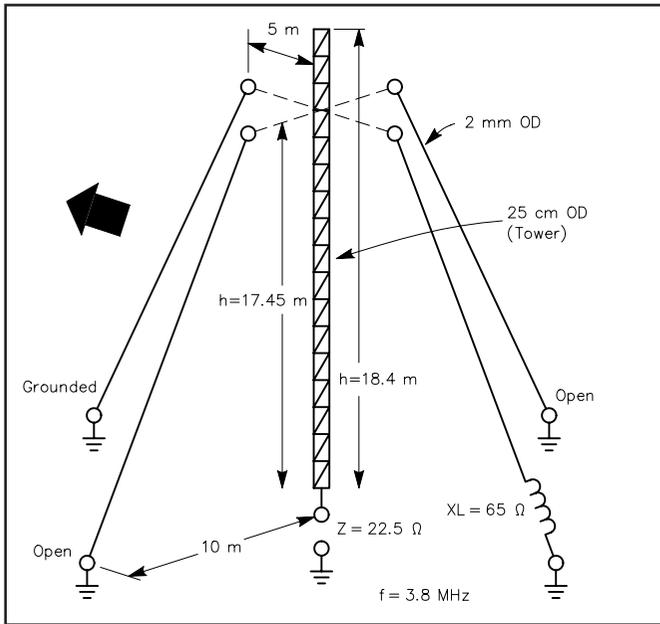
Figure 9—A three element array.
